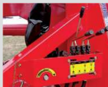
Independent Hydraulic Controls. Speed Control Valve.
